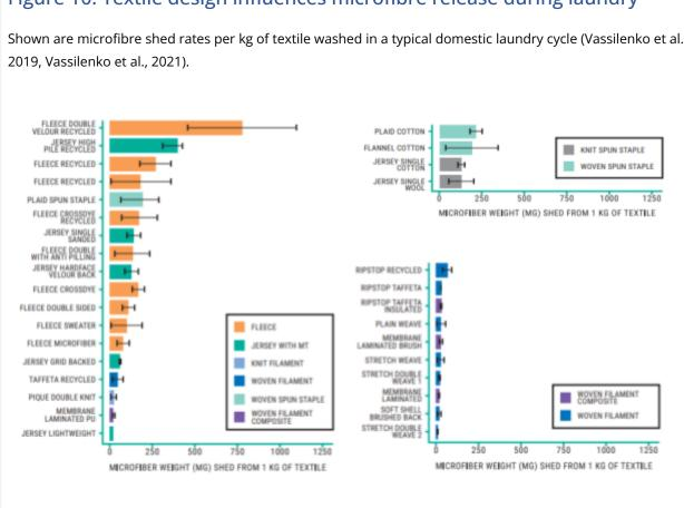
Figure 10. Textile design influences microfibre release during laundry
